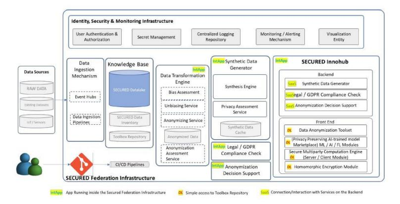
The broader **SECURED** architecture contains several interconnected services which cooperate to provide the overall platform functionality. Purely from an architectural standpoint, these services are contained inside the **SECURED Federation Infrastructure**, more or less an umbrella-entity that allows us to define the boundaries of the provided solution as well as to properly identify the necessary communication interfaces and flows that need to be implemented.
